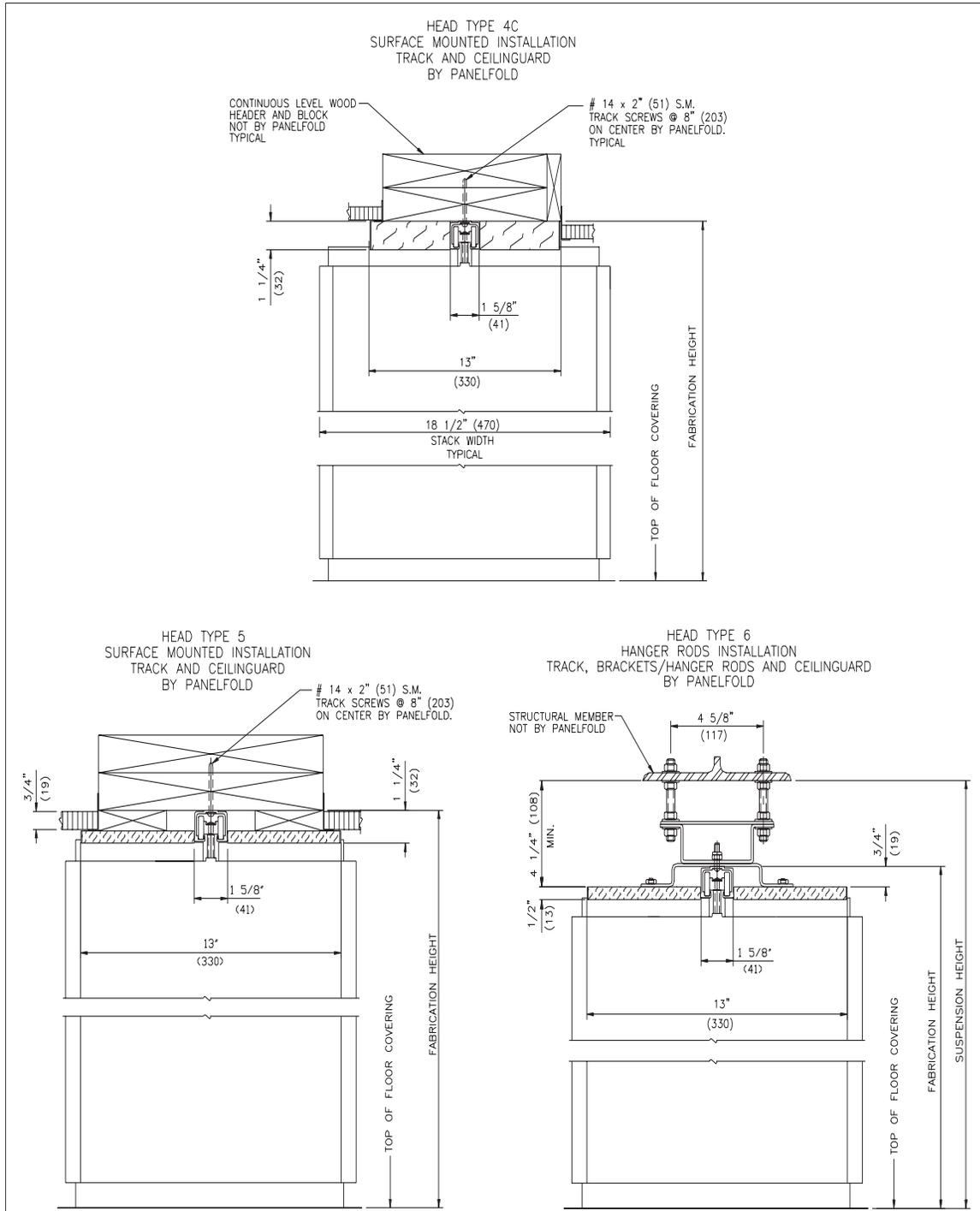
All dimensions shown in parentheses are millimeters. Scale: N.T.S.
