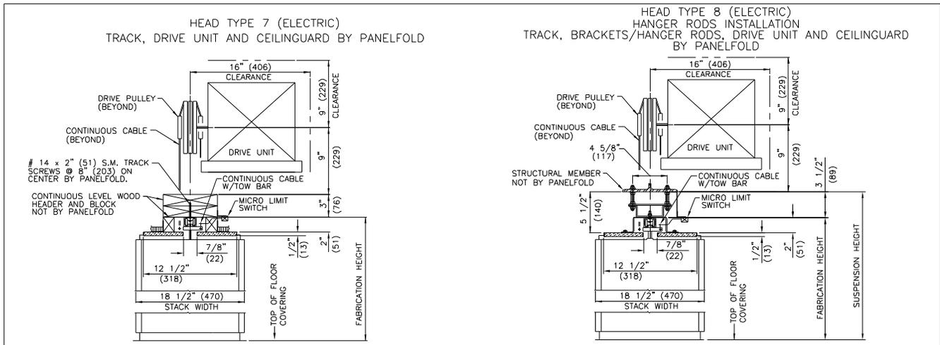
All dimensions shown in parentheses are millimeters. Scale: N.T.S.
