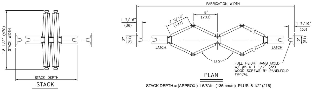
All dimensions shown in parentheses are millimeters. Scale: N.T.S.
